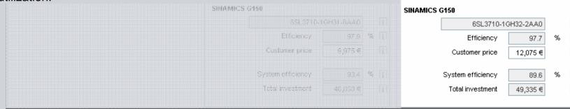
805 gearbox – N-compact – SINAMICS G150 Gear i Coupling gearbox - load 1,200€ i Gear efficiency 96.0 % i Transmission ratio i 1:7.4 i Customer price gear 12,400 € Coupling motor - gear i 300€ Induction motor i 1PQ83154PM80 -ΚW i Rated power 235 95.5 % i Efficiency i Required current 178 A i Customer price 23,360 € i i i i i
